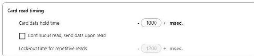
The screenshot shows a configuration window titled "Card read timing". It contains three settings: "Card data hold time" set to 1000 msec, "Continuous read, send data upon read" which is unchecked, and "Lock-out time for repetitive reads" set to 1200 msec.
